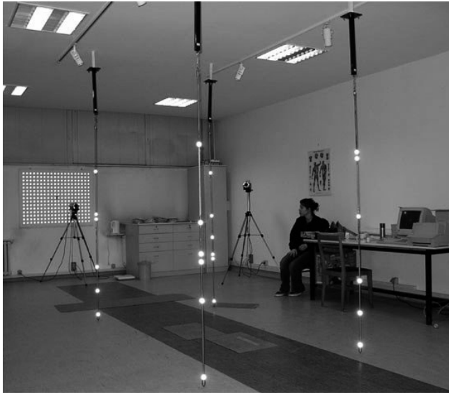
Figure 7. Example of a modern gait lab, with 3D vicon and a forceplate.
